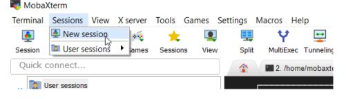
8. It will pop a new window, in that select SFTP, on remote host fill the IP address that was assigned to the board, on user name in this case is root, and the click OK:
