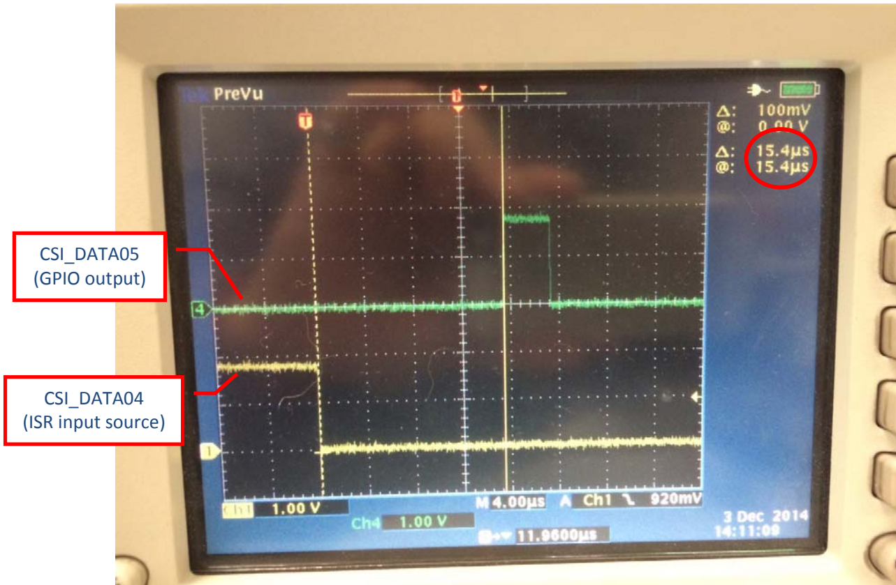
Figure 1. 15.4us is the time gap between external H/W GPIO interrupt pin and the start of the execution of the first useful instruction in ISR.
