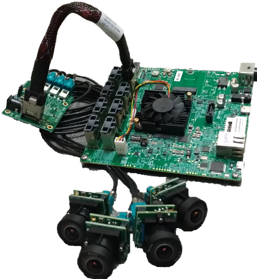
Figure 12. i.MX 8QM MEK 4 cameras example
