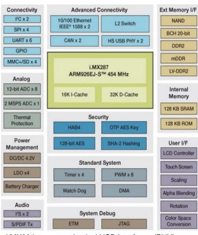
i.MX28 integrates physical USB interfaces (PHY), 10/100 Ethernet , power management, and a resistive touch screen display controller.
