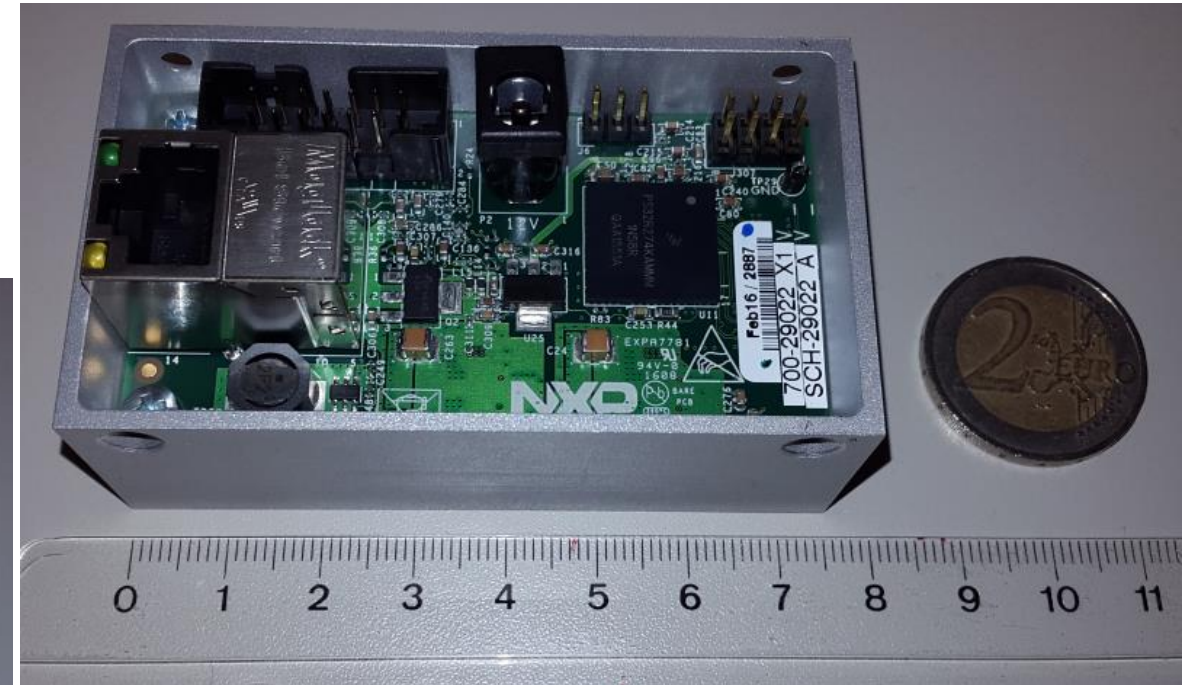
Back side, RRU with debug and Ethernet:
