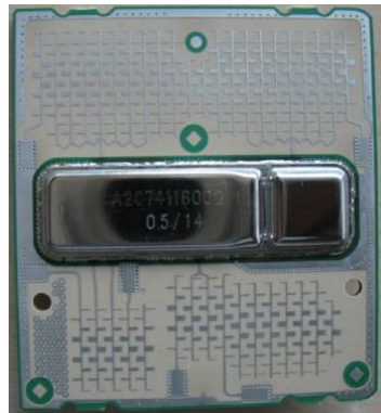
NXP MR2001 Scalable radar transceiver chipset with antenna arrangement
