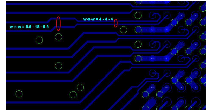
Figure 4. Optimum Layer Assignment for Effective Backdrill
