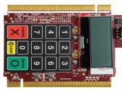
The TWR-PoS-K81 development platform is a reference platform for a payment pin entry device. This board includes Cirque SecureSense AFE for secure pin entry. The design files and associated software show an example pin pad application that has been submitted for Payment Card Industry certification. The board is designed to work standalone or as part of the NXP Tower System.
