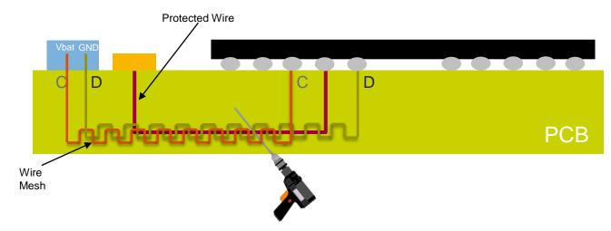
DRYICE module will detect Tamper and initiate key erasure when:
