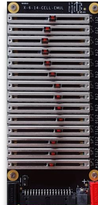
14-Cell Isolated Pack emulator (in Development)
