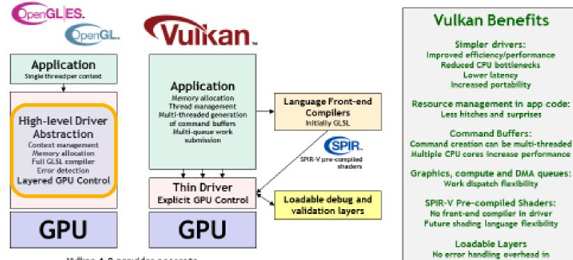
Vulkan 1.0 provides access to OpenGL ES 3.1 / OpenGL 4.X-class GPU functionality but with increased performance and flexibility
