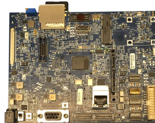
SCM6D running on a 14 Layer HVB running at 800MHz
