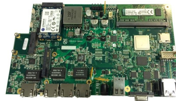
Discrete iMX6DQ with SoDIMM DDR3, 8 Layer, running at 1GHz
