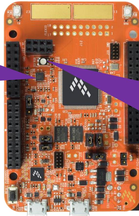
Building from a KSDK example, FlexIO emulates an I2C master to collect data from the 6 axis sensor
