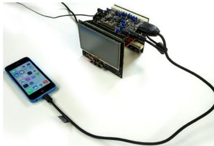
iPhone, iPad or iPod connected to Tower system via TWR-DOCK2 and custom Lightning or 30-pin connector cable
