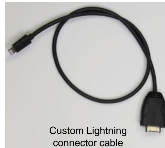
iPhone, iPad or iPod connected to Tower system via TWR-DOCK2 and custom Lightning or 30-pin connector cable
