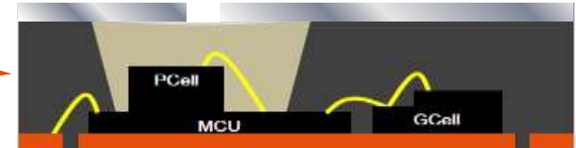
QFN 7x7 Cross-section illustration
