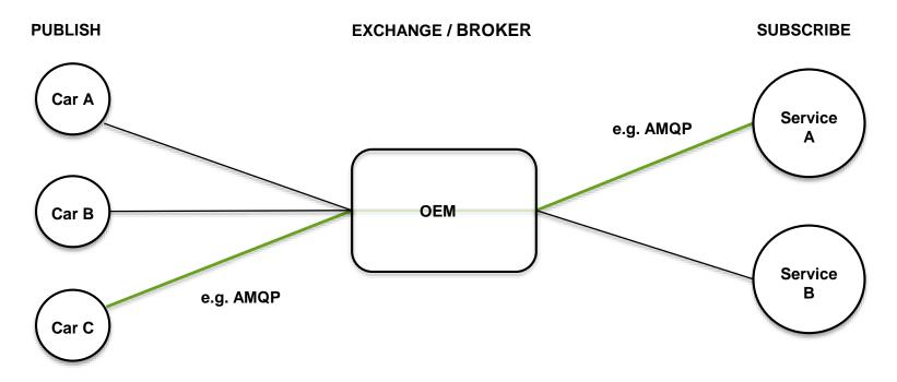
Two related exchanges, automatically connected & triggered by broker
