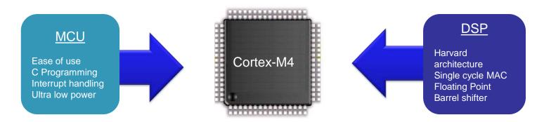
The Cortex-M4 is ~2X more efficient on most DSP tasks than leading 16- and 32-bit MCU devices with DSP extensions
