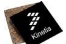
143WLCSP 6.5x5.6x0.56 mm 0.4mm pitch (K61)
