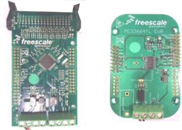
High voltage battery management system Freedom Platform + MC33664 + daisy chain MC33771
