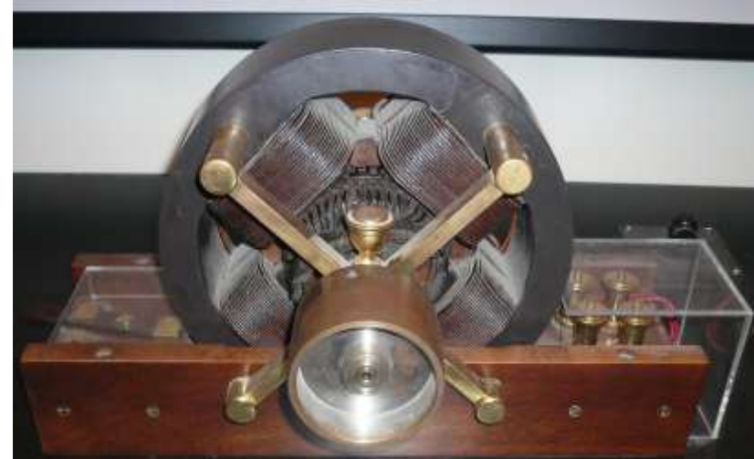
Model of Tesla's 1 st Induction Motor Demonstrated 1885
