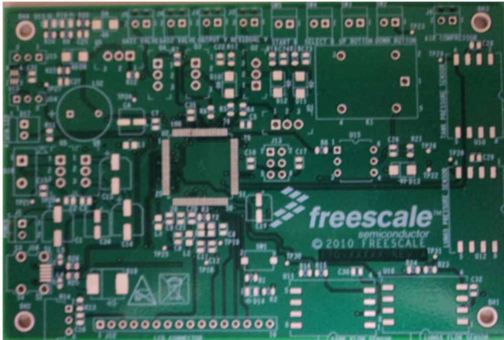
Figure 4-19. Ventilator PCB top view without components
