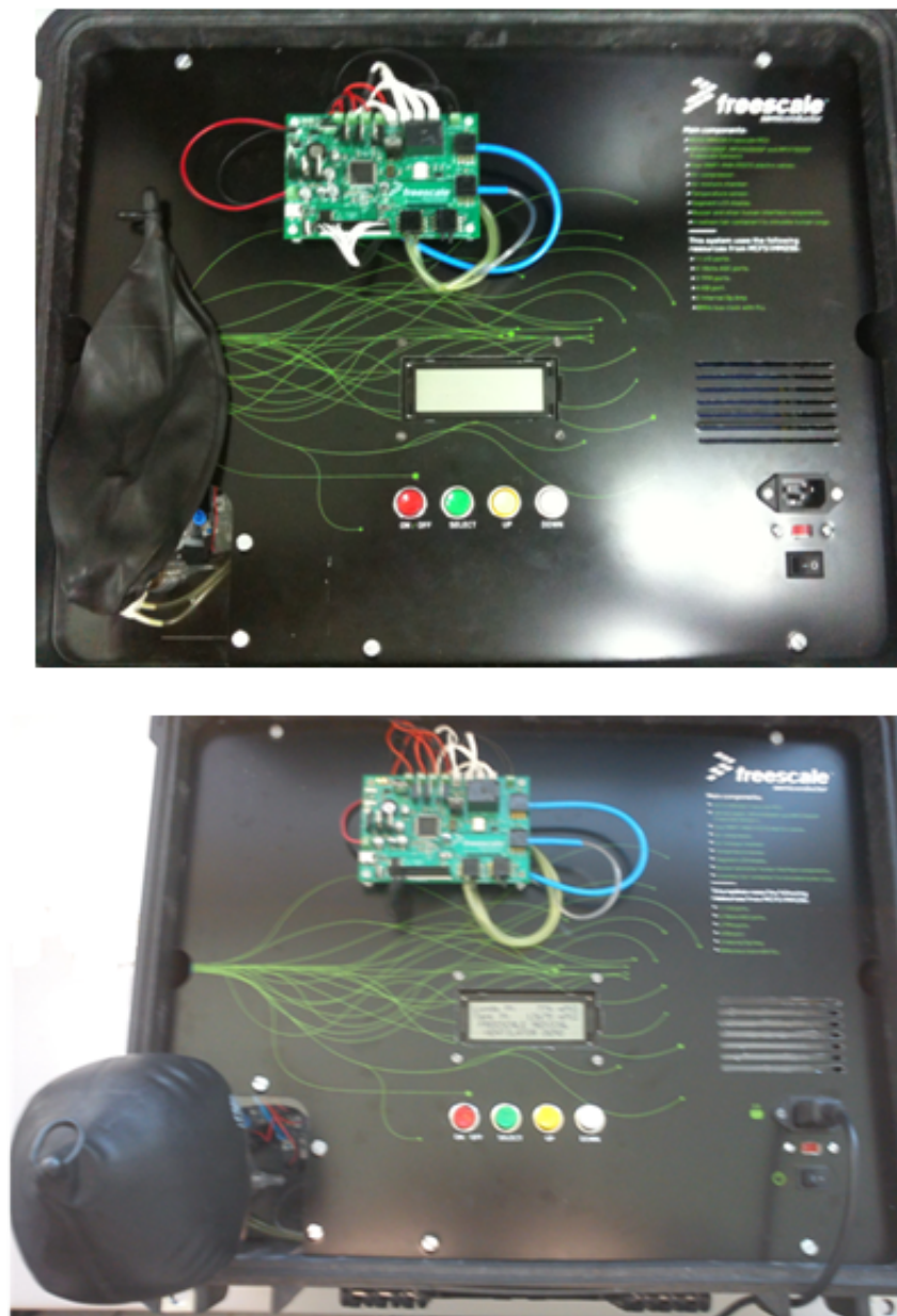
Figure 4-24. Ventilator front panel
