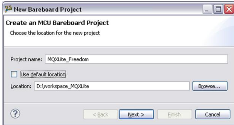
Figure 10. New project wizard – Name and Location
