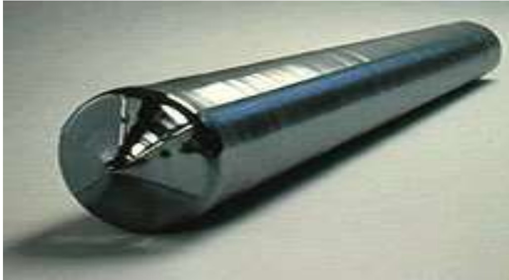
Single crystal silicon ingot length: 110 cm
