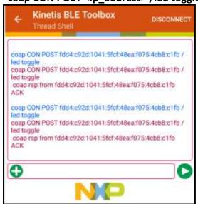
19. Run the command a few more times to make the LED on R2 toggle on and off via the BLE app. Make use of the **Shortcuts** and **Recent** buttons in the app to save some time typing. You can also try getting the temperature like you did in the previous lab.
