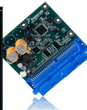
Airbag Reference Design
