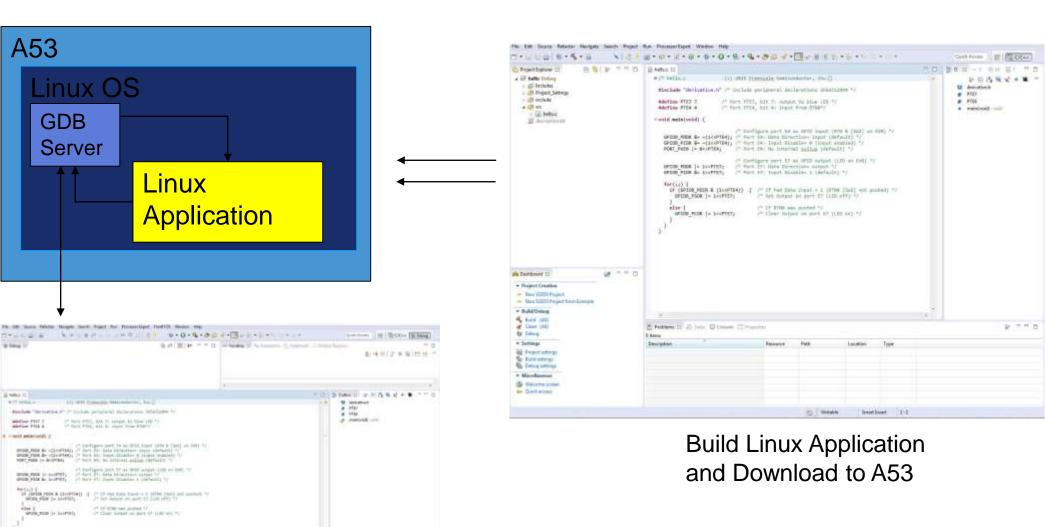
Debug Linux Application on A53 In S32 Design Studio through GDB server in Linux OS
