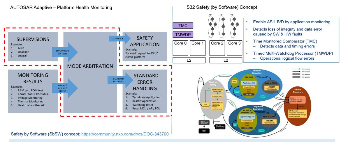
NXP's Safety Concept with the patented Safety by Software (SbSW) method, for performance cores, to efficiently enable the AUTOSAR Classic and Adaptive Platform Heath Monitoring & Safety.
