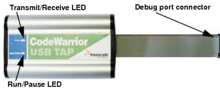
Figure 4-1. USB TAP probe - top view
