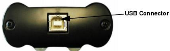
Figure 4-2. USB TAP probe connector - end view
