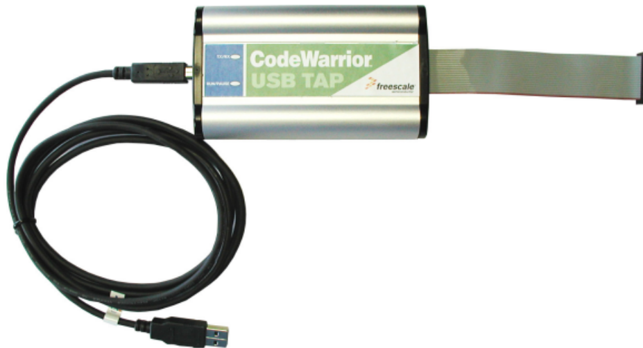
Figure 1-1. USB TAP probe with USB 2.0 cable
