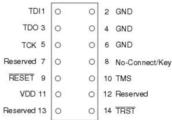
Figure 8-1. USB TAP probe for OnCE connector pin assignments
