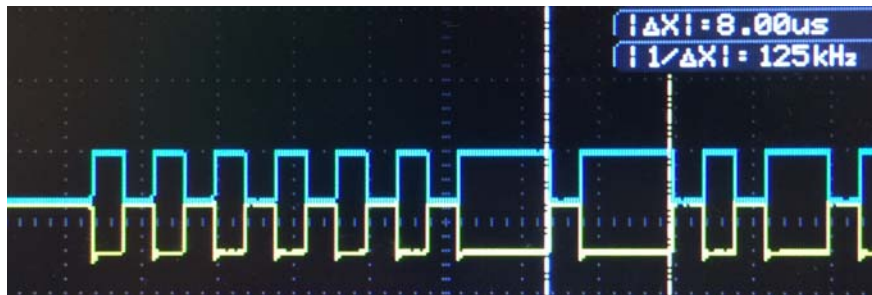
Figure 14. CANH, CANL at start of CAN 2.0 transmit frame with standard ID 0x555
