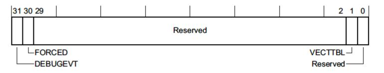
**DEBUGEVT** - Indicates that a debug event occurred while the debug subsystem was not enabled
