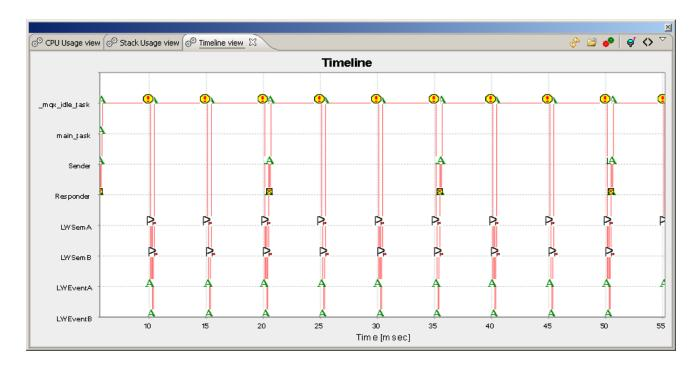
The graph shows task switches in your application. Icons represent various events logged by the MQX kernel such as interrupts, synchronization calls, message sending, etc.
