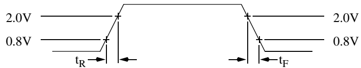
FIGURE 7. Input/Output Valid Level for AC Measurements
