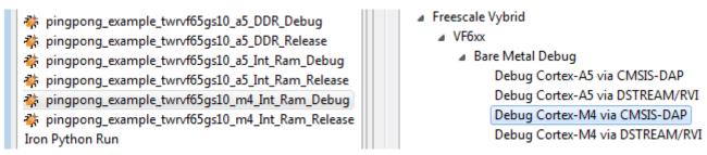
The Cortex-M4 project will be loaded to the device and execution will stop in the main () function. Press the *Run* button to continue in the *pingpong\_example\_twrvf65gs10\_m4* program execution.
