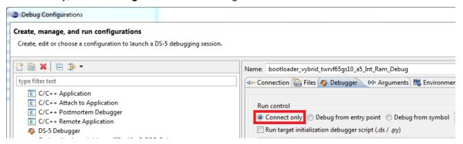
The debugger will connect to the selected application. You can stop the selected core and debug the booted image.
