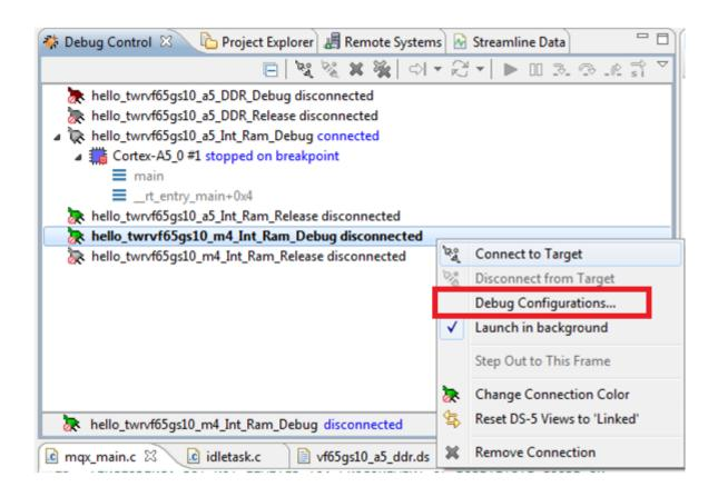
• Select **Debug Configurations** and verify that the **Enable Cortex-M4 clock** option in the **DTSL Options** menu is still checked.
