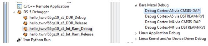
• The Development Studio 5 (DS-5) will switch to Debug Perspective automatically. Then, the project will be loaded to the device and execution will stop in the main() function.
