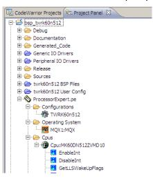
• Right click the CPU and select "Inspector". The CPU Component Inspector opens.
