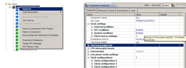
• Unfold the "Internal oscillator" item and set the required parameters.
