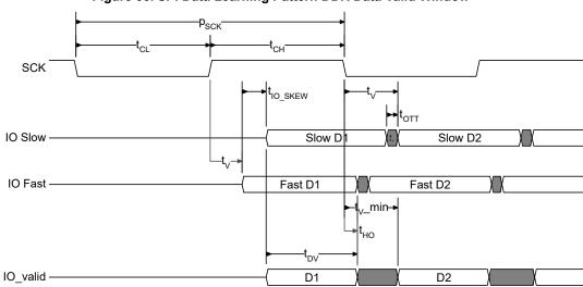
The minimum data valid window (t<sub>DV</sub>) and t<sub>V</sub> minimum can be calculated as follows:
