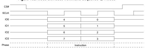
Figure 102. Mode Bit Reset Command Sequence QPI Mode
