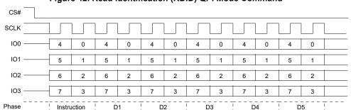
Figure 42. Read Identification (RDID) QPI Mode Command
