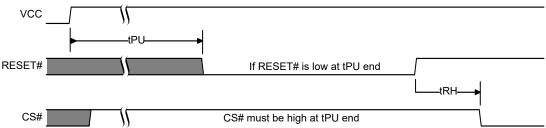
Figure 24. Reset HIGH at the end of POR
