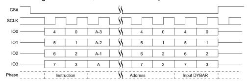
Figure 92. DYBWR QPI Mode Command Sequence<sup>[59, 60]</sup>
