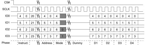
Figure 68. Quad I/O Read Command Sequence (4-Byte Address, ECh or EBh [CR2V[7]=1])
