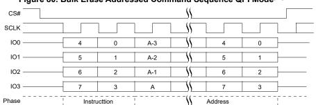
Figure 80. Bulk Erase Addressed Command Sequence QPI Mode<sup>[55]</sup>
