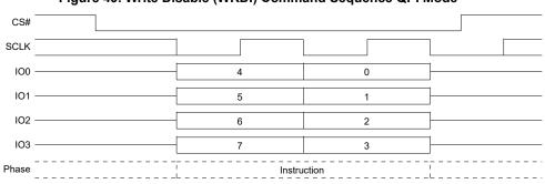
Figure 49. Write Disable (WRDI) Command Sequence QPI Mode
