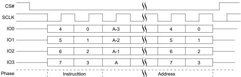
Figure 76. Parameter Sector Erase (P4E 20h or 4P4E 21h) QPI Mode Command Sequence<sup>[53]</sup>
