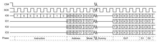
Figure 71. DDR Quad I/O Read Initial Access (4-Byte Address, EEh or EDh [CR2V[7]=1])[49]
