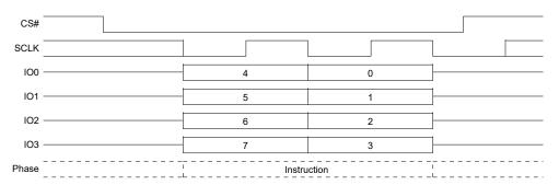
Figure 104. DPD Command Sequence QPI Mode
