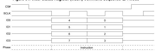
Figure 51. Clear Status Register (CLSR) Command Sequence QPI Mode
