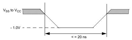
Figure 17. Maximum Positive Overshoot Waveform
