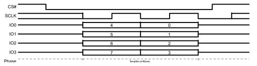
Figure 100. Software Reset Command Sequence QPI Mode
