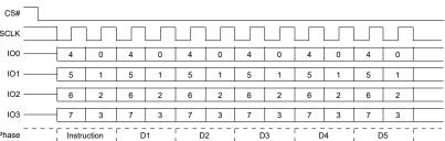
Figure 43. Read Quad Identification (RDQID) Command Sequence
