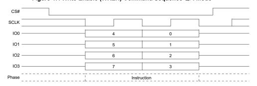
Figure 47. Write Enable (WREN) Command Sequence QPI Mode
