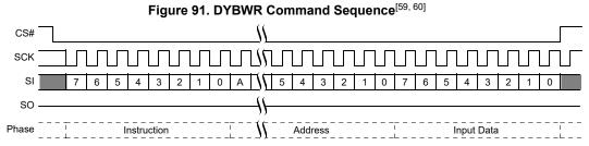
This command is also supported in QPI Mode. In Quad All Mode, the instruction is shifted in on IO0-IO3, two clock cycles per byte.
