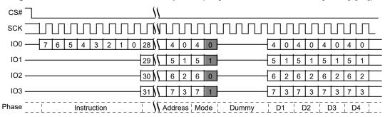
Figure 69. Quad I/O Read Command Seq. (4-Byte Address, ECh or EBh [CR2V[7]=1]) QPI Mode
