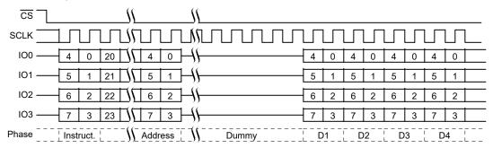
Figure 54. ECCRD (19h), Quad All Mode, CR2[7] = 1, or 4ECCRD (18h) Command Sequence
