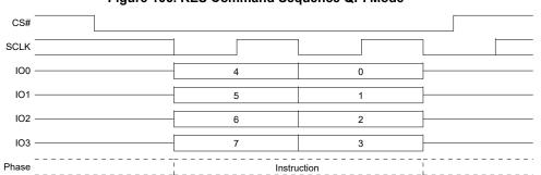
Figure 106. RES Command Sequence QPI Mode
