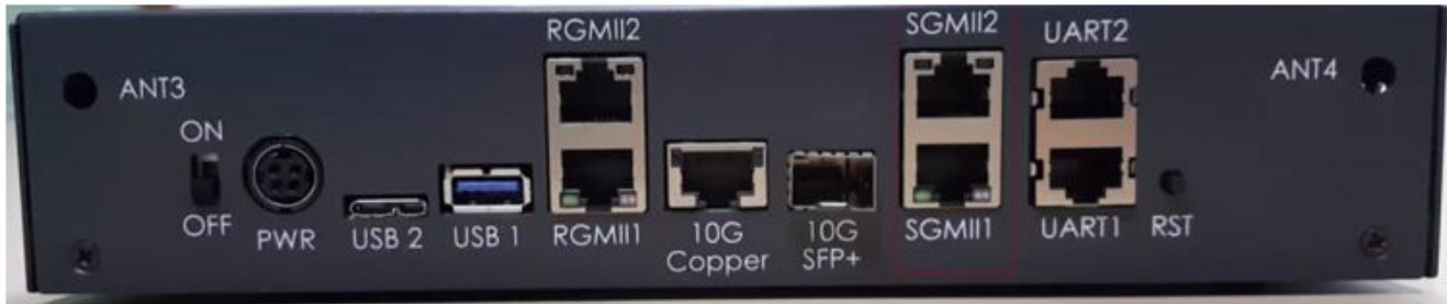
Figure 201. LS1046ARDB Port Layout
