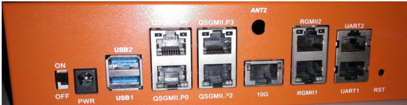
Figure 199. LS1043A Port Layout
