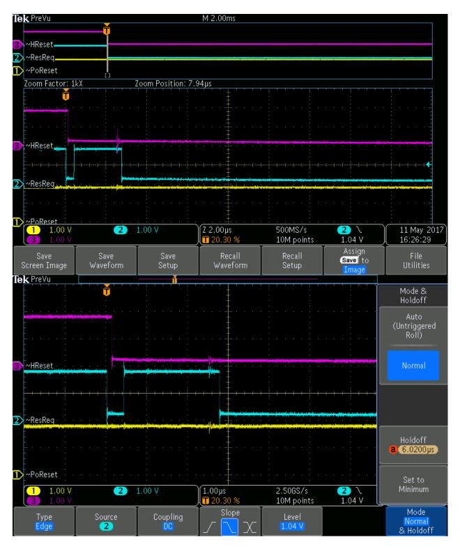
In this case the ~RESET\_REQ initially looks like before (SDHC case) but 2.36uS after deasserting it drives low again. This condition persists forever. We have tried masking all the ~RESET\_REQ sources in the RSTRQMR1 but the failure is the same.
