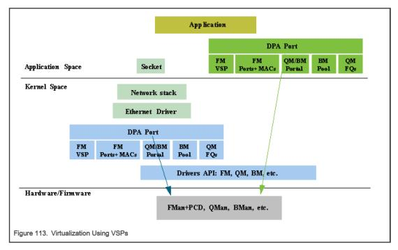
The global FMan module is in charge of the Virtual Storage Profiles entries management. On FMan initialization, the first VSP index dedicated to this partition must be defined (it should be an absolute index), and so is the total number of VSP's for this partition. Later, for each port using VSP's, a window of entries should be defined. VSPs may not be shared among FMan
