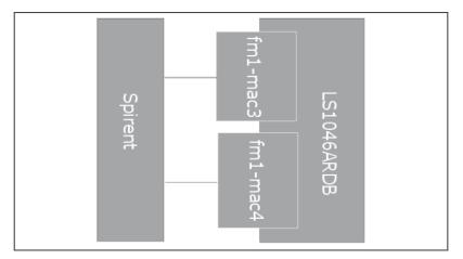
In the above figure, an NXP LS1046ARDB board is shown connected to a packet generator (Spirent). The example uses Spirent as packet generator, however, any other source of controlled packet transmission can also be used. The figure uses fm1-mac3 and fm1-mac4 interfaces for demonstration.
