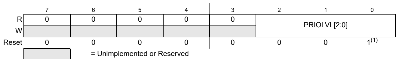
Figure 4-10. Interrupt Request Configuration Data Register 5 (INT_CFDATA5)
