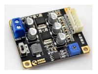
Power supply module Responsible for the entire system power supply, can provide multiple power supply,ensure the 3.3V system power supply, 5V system and the steering gear power supply requirements.
