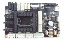
Main control board Responsible for the entire system of external signal input and human-computer interaction,multi-machine communication, servo control.
